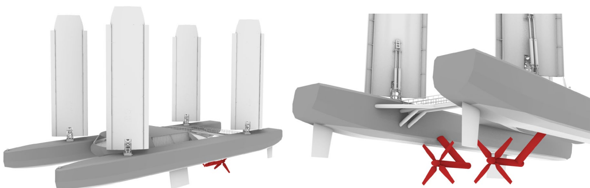
Figure 1. Conceptual 3MWe vessel diagram. 70m LOA, 4x250sqm wing sails, 2x5.5m hydrokinetic turbines (red).
